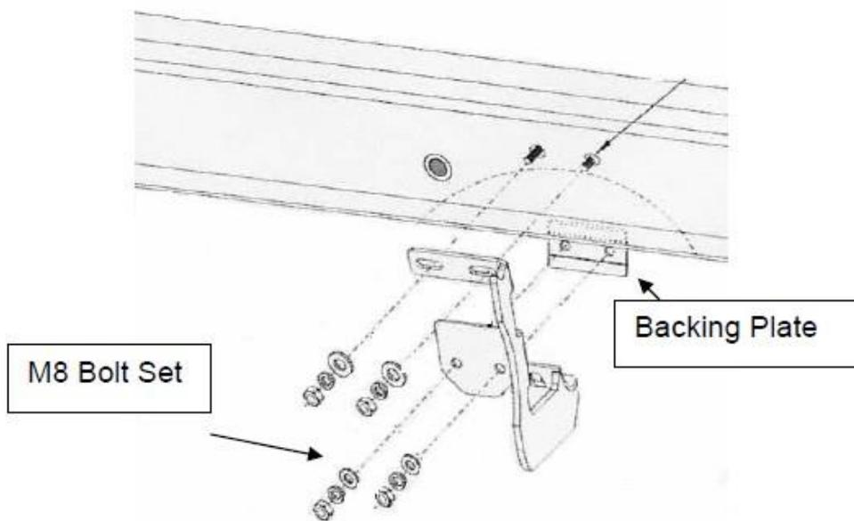
Figure 2. Passenger Side Center Bracket
