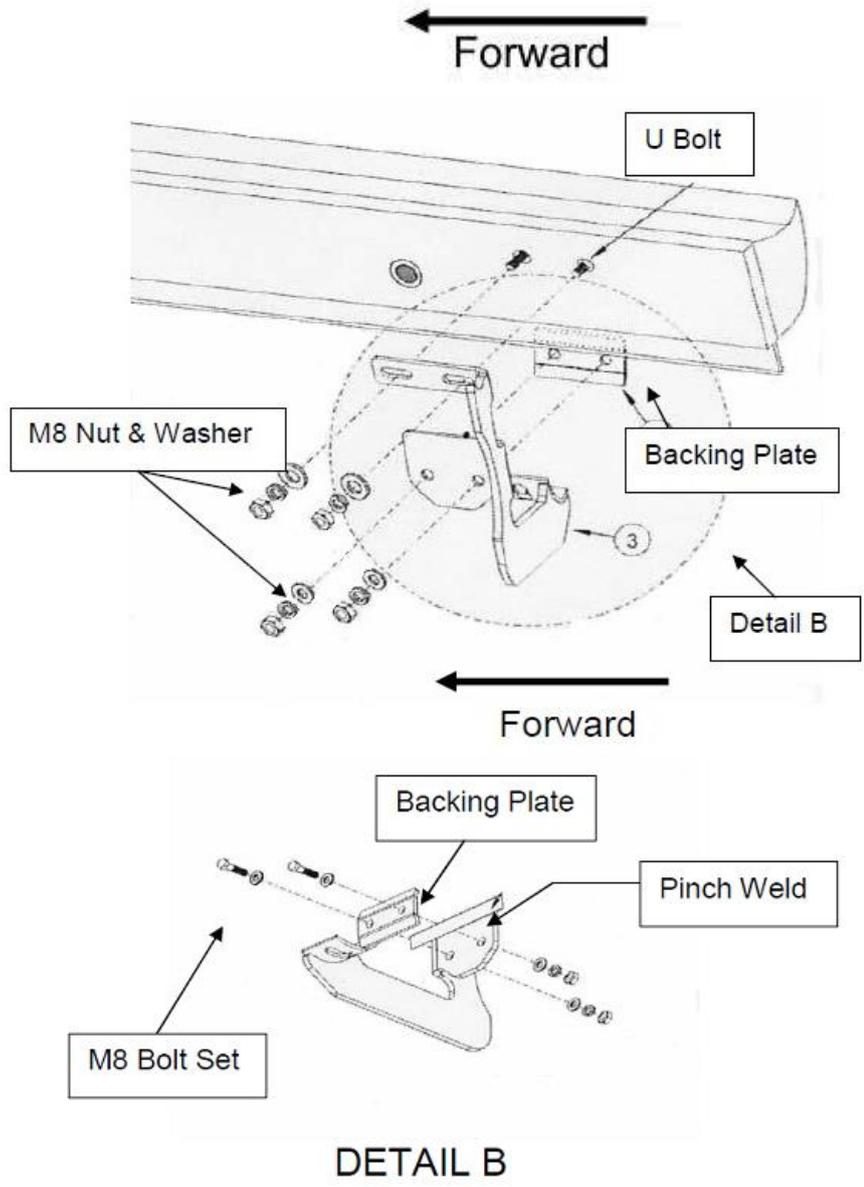
Figure 3. Passenger Side Rear Bracket
