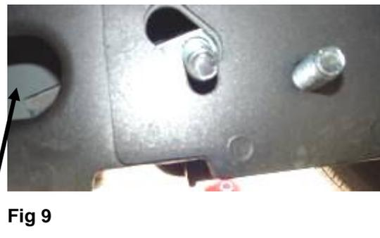
Driver's side front bracket attaches to bolt plates shown to the right.
