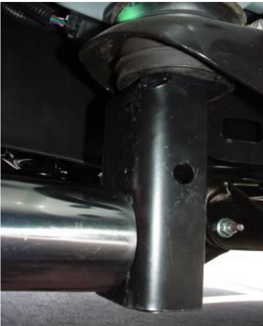
Hook front auxiliary bracket to inside of Rocker panel just like the rear.
