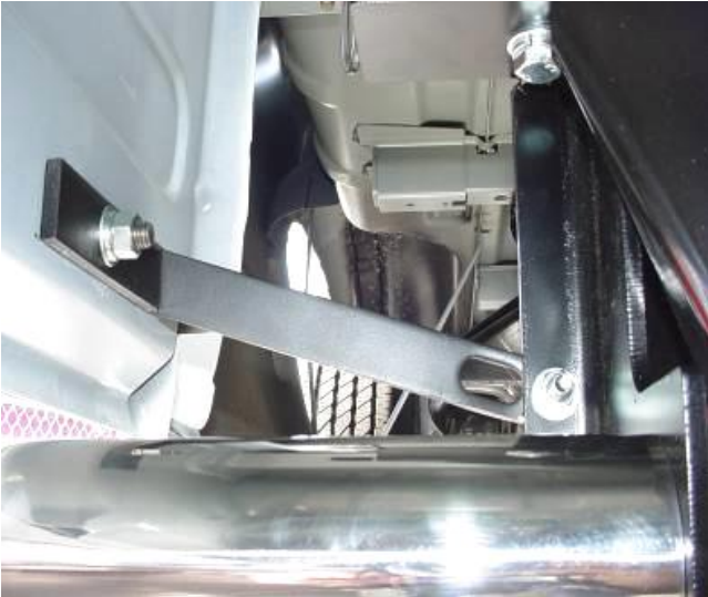
Passenger Side Rear Main Bracket and Rear Auxiliary Bracket (Looking towards rear of truck).
