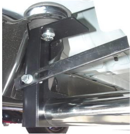
Passenger Side Rear Main Bracket and Rear Auxiliary Bracket (Looking towards front of truck).
