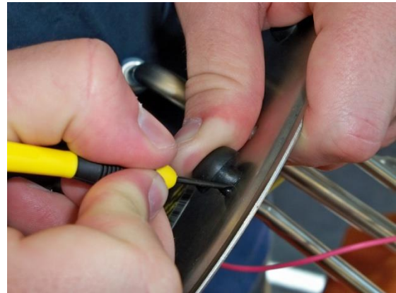
(Fig. 4) Gently and carefully “tuck” edge of the plug into the hole.
