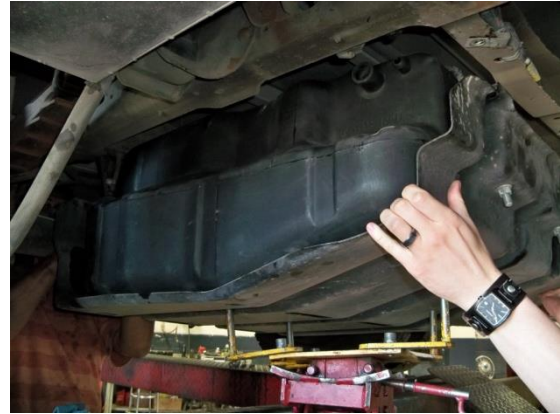
(Fig. 14) Lift tank into vehicle.
