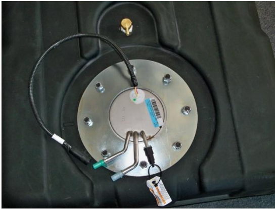
(Fig. 13) PS-191 Sending Unit Installed in TITAN tank.
