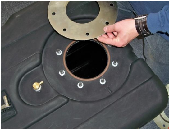
(Fig.9) Place one adaption flange on top of the tank's sealing "O" ring.
