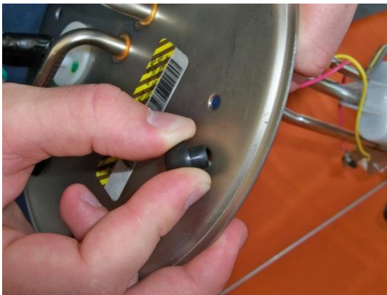
(Fig. 3) Work plug into the hole.
