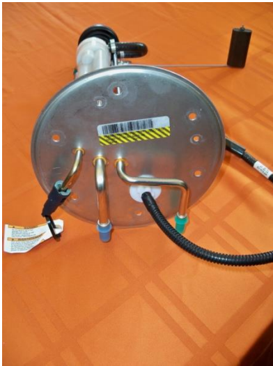
(Fig. 1) PS-123 Sending Unit mounting plate, showing bolt holes to be plugged.
