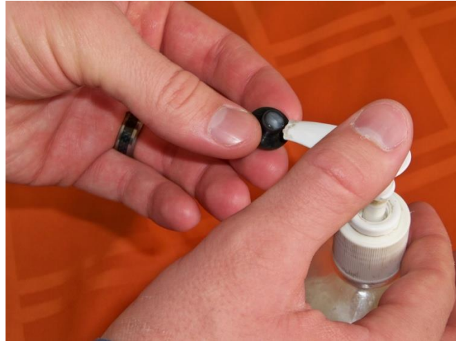
(Fig. 2) Place small amount of liquid soap on the tip of the nitrile plugs.
