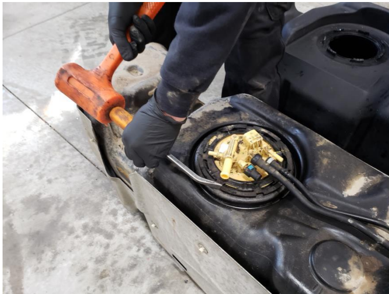
Sample image of removing an OEM lock ring
