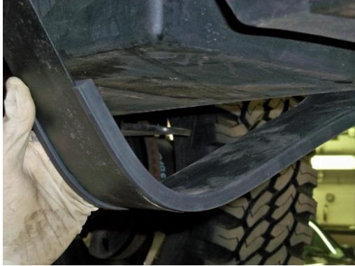
(Fig. 4) Install rubber bushings (pn 99 0000 0103) on both straps with the channel side toward the strap.
