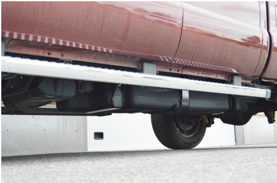
(Fig. 11) Completed front support installation and tank.
