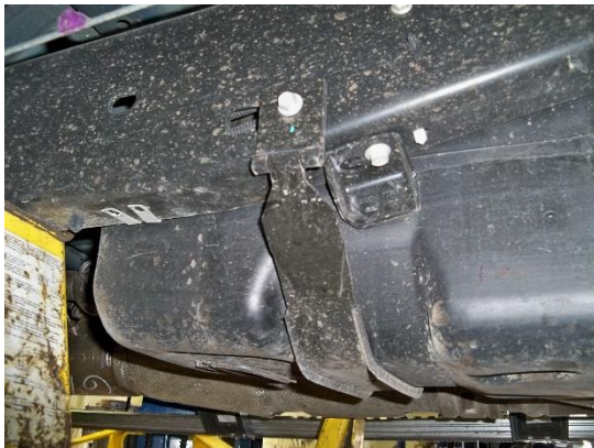
(Fig. 1) Remove original equipment strap and "bumper bracket", shown here to the right-hand side of the front strap.
