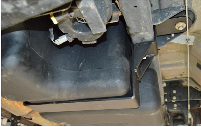
(Fig. 11) Completed front support installation and tank.
