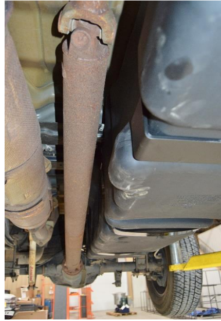
(Fig. 12) Installed front support on tank.
