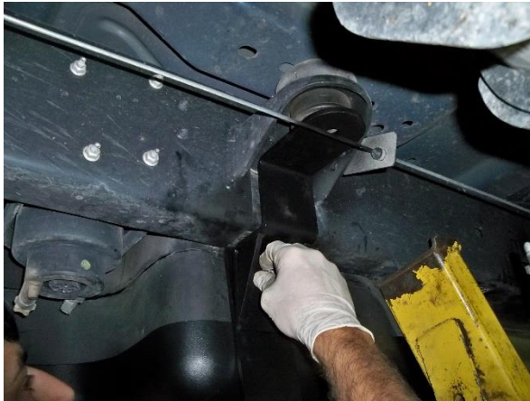
(Fig. 9) Mount the upper piece of the assembly to the lower piece using bolt provided.
