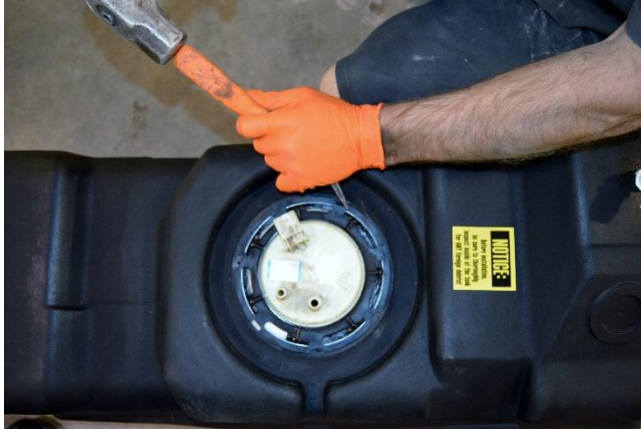
(Fig. 5) Using a hammer and punch, or screw driver to tighten the hold-down ring clockwise.
