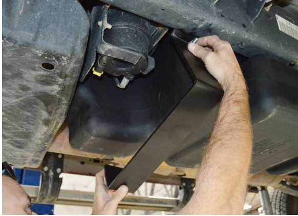
(Fig. 7) Hang lower piece of support assembly on lower lip of vehicle frame and slide towards the rear of vehicle until it lines up with cab mount.
