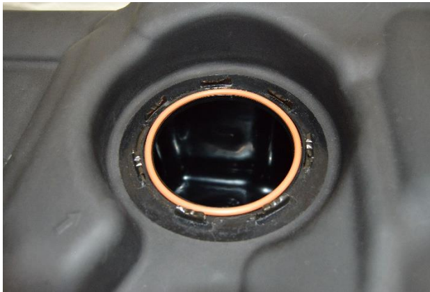
(Fig. 3) O-Ring gasket shown installed correctly.
