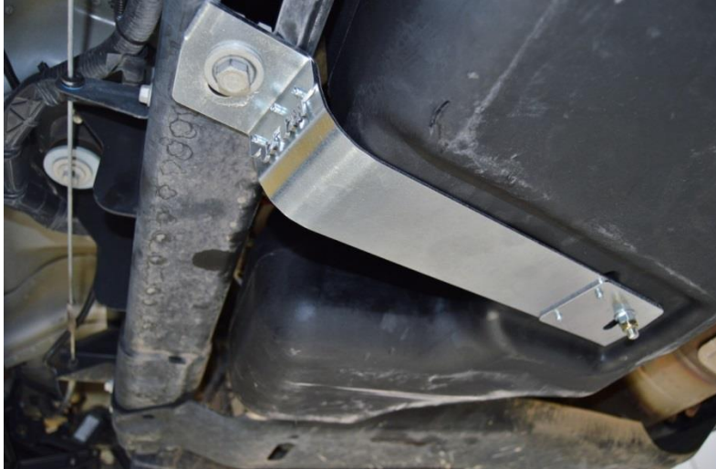
(Fig. 18) Front Support Assembly properly installed.
