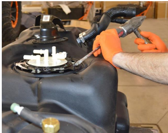
(Fig. 14) Reuse the OEM hold-down ring to mount the sending unit in the TITAN tank. Tighten by turning it clockwise as far as it will go.
