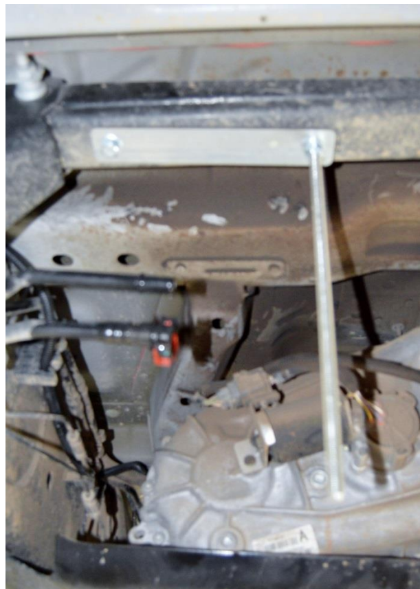
(Fig. 15) Partially assembled Front Support Assembly installed on the vehicle's cross member.
