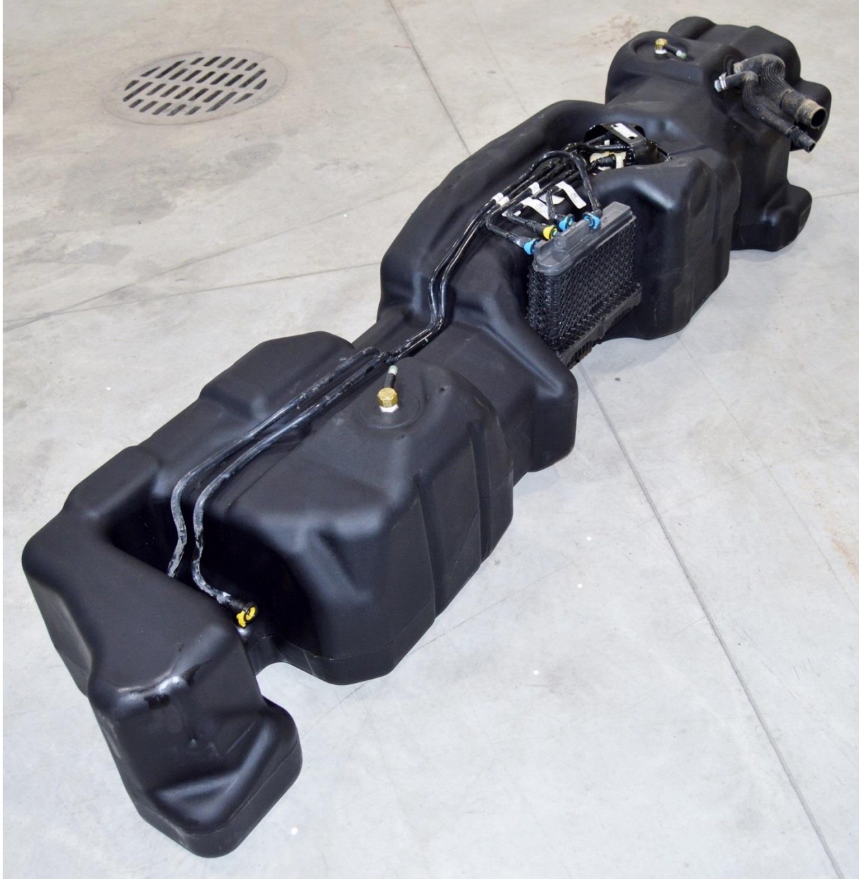
(Fig. 16) TITAN 7020317 tank shown with sending unit, water separator, fuel lines, sending unit guard, and fill and vent hoses installed; ready for installation into the vehicle.
