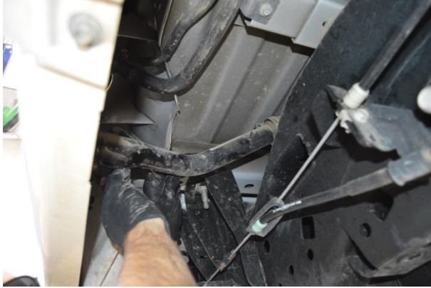
(Fig. 3) Move fill spout assembly toward vehicle frame to gain access to the hose clamps.
