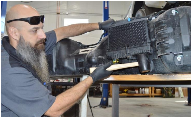
(Fig 10) Using a rubber mallet, carefully tap the water separator up and out of its mounting bracket on the OEM tank.
