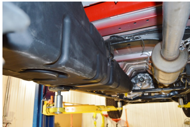
(Fig. 14) Inboard side view of the installed tank before the propeller shaft is reinstalled.
