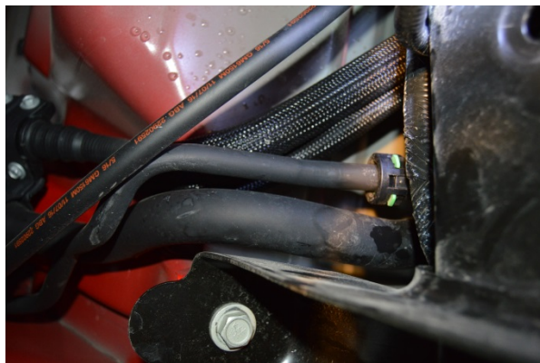
(Fig. 3) Primary vent line from the fill spout is accessible from the driver's side, underneath the vehicle. The quick connect coupling is shown with the green tabs.
