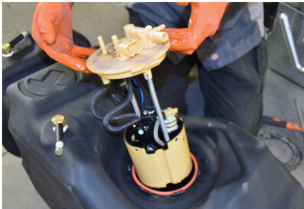
(Fig. 9) Remove the sending unit from the OEM tank. Remove the OEM O-ring, and place the sending unit into the TITAN tank as shown above.
