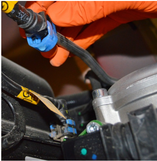
(Fig. 5) The two fuel lines at the front of the tank are shown here. The feed line is shown with the blue clip undone. To release these couplings, spread the blue tabs, as shown, and push them away from the lines.
