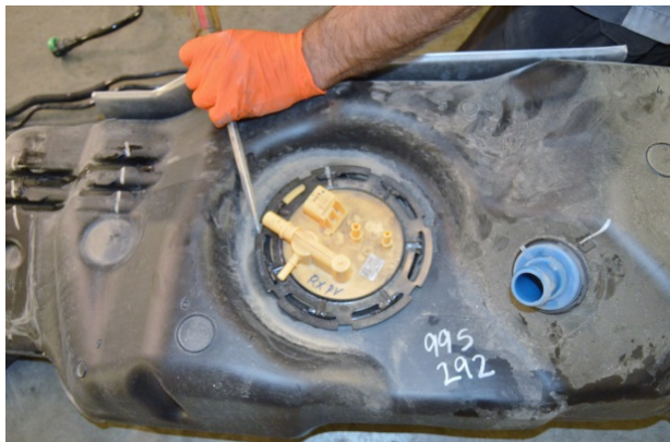
(Fig. 8) Loosen the hold-down ring on the OEM tank by turning counter-clockwise. Save the hold-down ring (Torque Ring), it will be reused on the TITAN tank.
