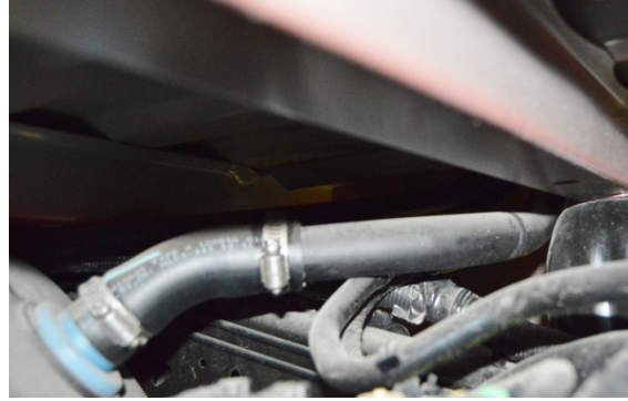
(Fig. 2) Loosen the clamps on the fill hose connected to the OEM tank's king nipple (shown here). Disconnect the fill hose from the OEM tank.
