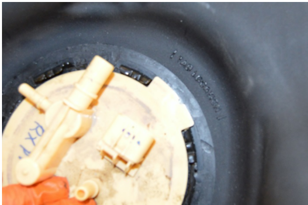
(Fig. 10) Be sure the tab on the sending unit lines up with the "TAB LOCATION" marks on the tank body as shown above.
