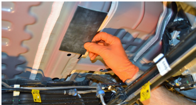
(Fig. 12) Remove the backing from the 3" x 6" EPDM Rubber Pad (pt. no. 01 0000 0147) and affix it to the underside of the cab near where the front of the TITAN tank will rest. Place as shown above.
