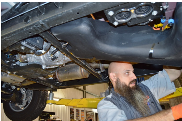
(Fig. 13) Angle the front of the tank up, over the tubular cross member which is just behind the transmission. Reconnect the front fuel lines before lifting the tank the rest of the way in.
