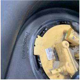
16 Place the top hold-down ring onto the lugs and the sending unit and turn it clockwise as far as it will go (see Fig. 5).
