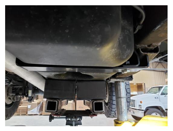
24 Insert 1-1/2" Fill Pipe ICV into the end of the fill hose with the "Flow" arrow pointing towards the fuel tank. This will need to be inserted deep enough to allow the fill hose to fit completely over the king nipple.
