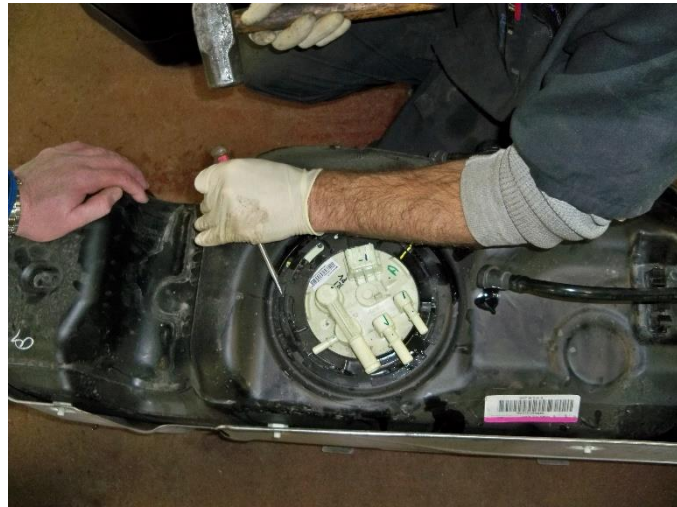
(Fig. 2) Loosen hold-down ring on OEM tank by tapping counter-clockwise, remove and lift out sending unit.
