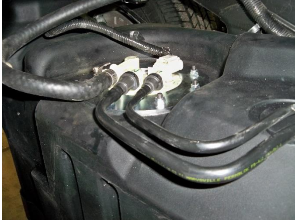
(Fig. 12) Lift tank high enough to reconnect electrical cable and vent hose to sending unit.
