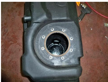
(Fig. 3) Leave the "O" ring gasket, studs and retainers assembled as they are (shown before sending
