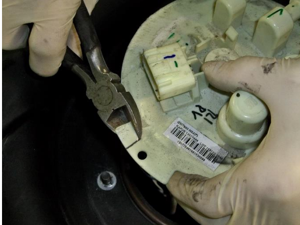
(Fig. 5) If sending unit connections interfere with the mounting studs, trim 1/2" off the side of the tab nearest the electrical connector.
