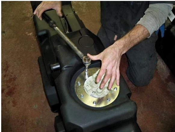
(Fig. 7) Using a torque wrench, tighten the top Flange nuts to 20 ft. lbs. using a “star” pattern.
