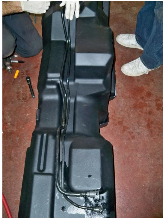
(Fig. 8) Attach the fuel lines to the sending unit and lay them in the retaining groove provided on the top of the replacement tank.
