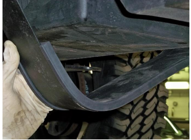
(Fig.13) Extruded bushings installed on straps
