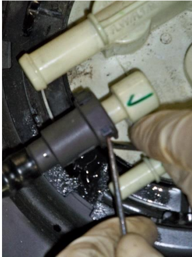
(Fig. 1) Disconnect fuel lines at the sending unit using pick.
