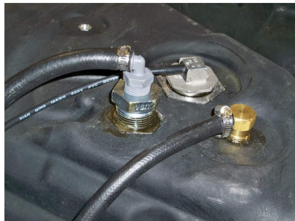
(Fig. 7) Install 5/16" hose onto the rollover valve as shown in this photo.
