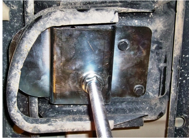
(Fig. 3) Cross member in 03-12 RAM vehicles showing STAFS Truck Mounting Plate close-up.
