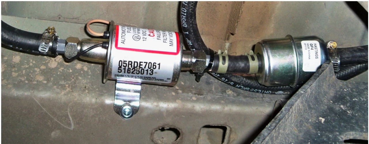
(Fig. 14) Fuel pump and inline filter installed.
