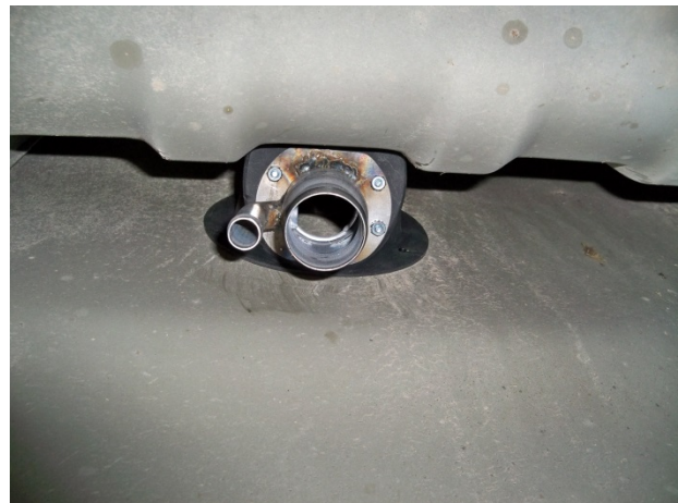
(Fig. 18) Check to be sure there is room in the fender space for the Poly Fuel Neck Flange Assembly BEFORE cutting any holes. Always test fit FIRST.
