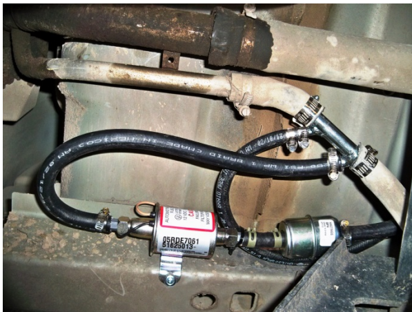
(Fig. 15) Vent Fill Neck Adapter installed.
