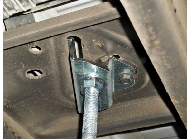
(Fig. 3) Cross member in 2011+ GM vehicles showing STAFS Truck Mounting Plate close-up.
