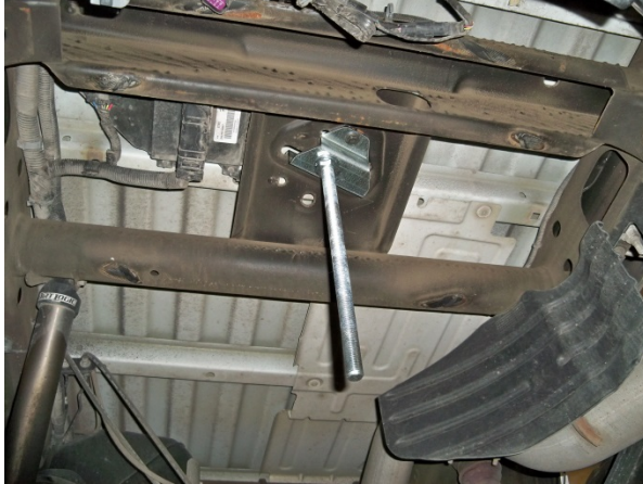
(Fig. 2) Cross member in 2011+ GM vehicles showing STAFS top Truck Mounting Plate and Threaded Rod installed.
