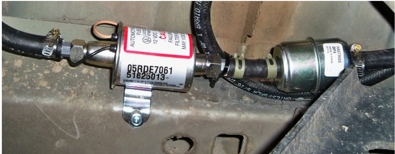
(Fig. 14) Fuel pump and inline filter installed.
