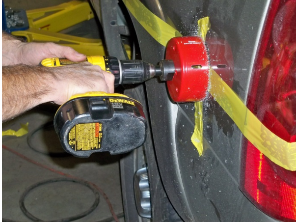
(Fig. 19) Use 4.75" hole saw to cut hole for Fuel Door.
