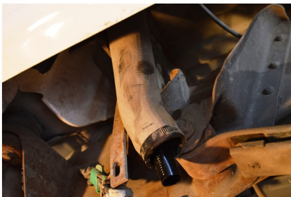
(Fig. 1) On vehicles with LB7 engines only, an interior fill hose is located inside the main fill hose. The tank vents through the space provided between the two hoses. Ten (10) inches needs to be cut off of the interior hose on end that goes to the tank as shown.
