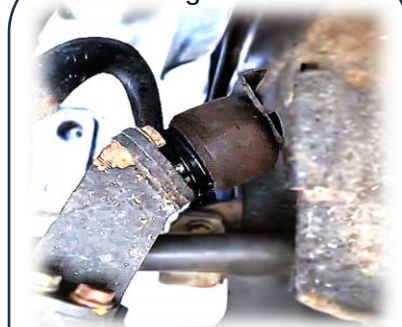
Ensure top rubber surface is flat with the landing part
