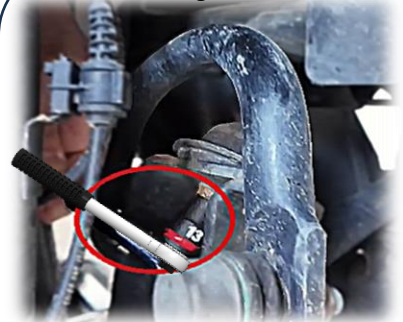
Use 13mm Socket for Easy Removal
