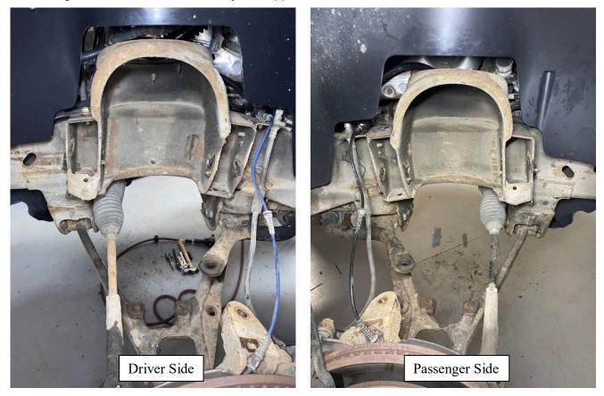
J. The upper control arm droop limiting bracket will need to be removed from the frame on both sides. Start by marking the cut line at the welds on both sides of the droop limiter as shown below. Then using a cut-off wheel, carefully cut the tab off of the frame.
