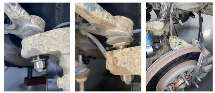
F. Using a 15mm wrench and socket, remove the sway bar link and lower shock bolts.
