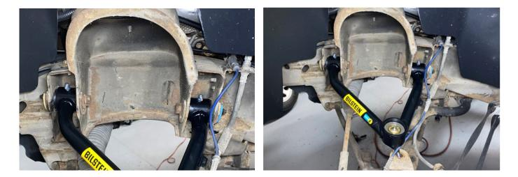
O. Reinstall the shock and spring assembly. Secure 3 top mount nuts using an 18mm wrench and lower mount using 15mm wrench and socket. Reattach the wiring harness clips to the top mount studs. Then reinstall the stabilizer link using a 15mm wrench and socket. Torque all hardware to OE specifications according to the manufacturer service manual.
