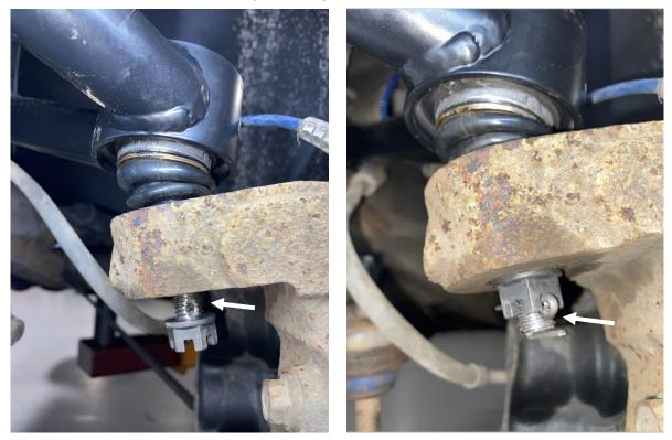
R. Using the supplied hose clamp, screw, locknut and 2 washers, secure the ABS line to the tab on the UCA as shown below. Using a 3/8" wrench and 1/8" allen, tighten the screw and nut, then verify ABS line has adequate slack to accommodate steering and suspension motion.
