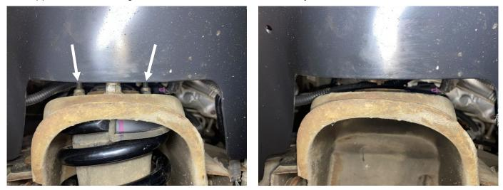
H. Using a 21mm wrench and socket, remove both cam bolts, then remove the OE upper control arm from the vehicle.
