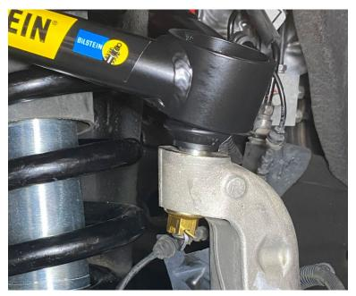
x. Reinstall the tie rod end to the spindle using a 21mm wrench and 10mm wrench. Then using a 10mm wrench, reinstall the brake line bracket and ABS line bracket to the rear of the spindle.
