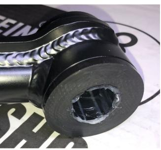
O. Press the steel sleeves into the bushings and apply more grease to outside faces of the bushings and sleeves.
