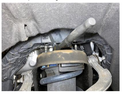
J. Remove the shock for access to the upper control arm bolts. Using a 21mm socket and 21mm wrench, remove the upper control arms.
