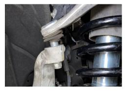
G. Remove the upper ball joint from the spindle and carefully secure the spindle using a bungee to avoid tension on the brake line and ABS line.
