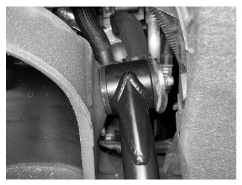
R. Apply non-permanent thread locker to the UCA bolts and install the flanged nuts. Torque bolts to 122 Nm (90 ft.-lbs.).
