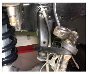
Using a 19mm socket and 19mm wrench, remove the nuts from both UCA pivot bolts. Leave the bolts in place at this time. Note that both UCA pivot bolts are facing forward toward the front of the vehicle with the head of the bolts on the rear side of the vehicle.
