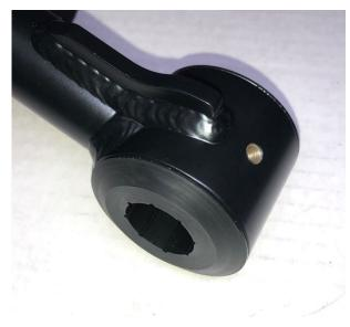
L. Apply the supplied grease to the bushing inside diameter.
