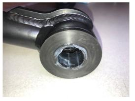
P. Press the steel sleeves into the bushings and apply more grease to outside faces of all bushings and sleeves.
