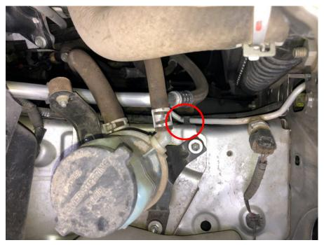
J. To allow removal of the UCA on both sides, remove the 2 clips that secure the smaller wiring harness to the inner fender.
