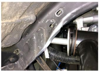
L. Carefully remove the UCA bolt. The UCA can now be removed. Save the UCA bolt and flanged nut as they will be reused later. The OE washers can be discarded.
