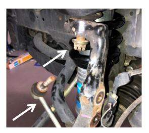
E. Using a ball joint puller, separate the spindle from the ball joint stem. Be careful to avoid tension on the brake line and ABS line.
