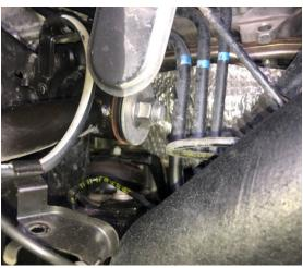
E. Remove cotter pin from upper ball joint castle nut. Using a 19mm wrench, loosen upper ball joint castle nut until flush with the end of the stud.
