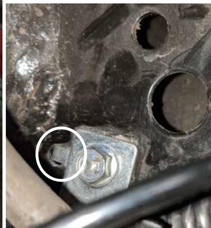
Figure 6. Breather hose bracket
