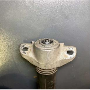
27. From the BILSTEIN rear parts kit, locate the support disc (item #7) to place on the mount tenon of the piston rod. Reassemble the OE top mount with Bilstein B8 Terrasport rear shock using the BILSTEIN Nyloc nut (item #6).
