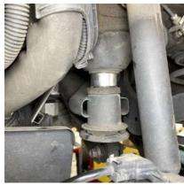
17. Following the factory service manual, torque all four bolts and both bracket nuts to OE torque specs.
