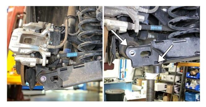
21. Lower the jack slowly to release the spring while preventing the spring from falling out.
