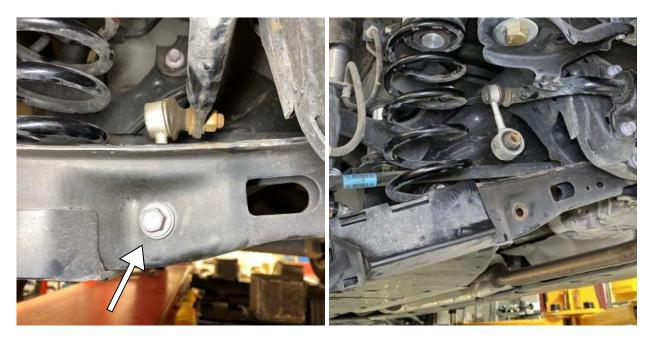
19. Note, or mark, the rear spring orientation at the upper and lower spring seats to ensure alignment for reassembly.
