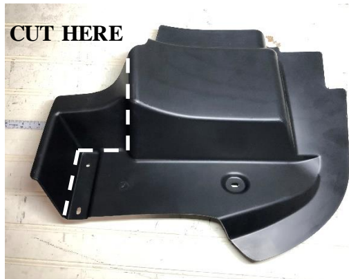
Figure 7 – Left Side Before Trimming
