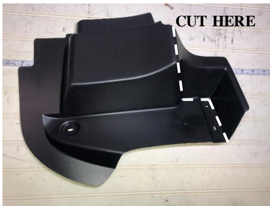
Figure 5 - Right Side Before Trimming
