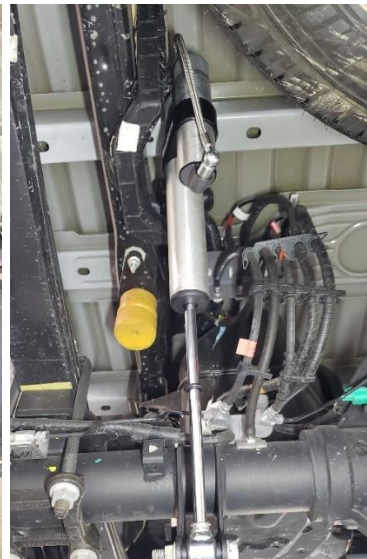
Figure 3. Rear Driver Side with wiring harness (View from rear)
