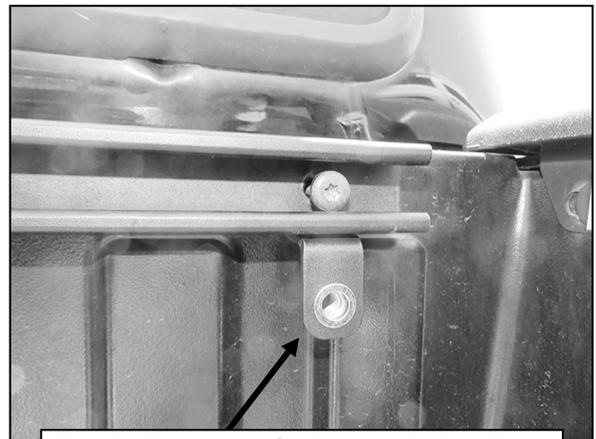
**(Fig 2) Reuse the factory bolts to attach the (5) Upper Mounting Brackets**
