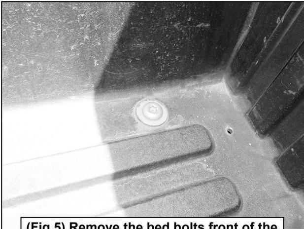
(Fig 5) Remove the bed bolts front of the bed, place the bolts in a safe location
