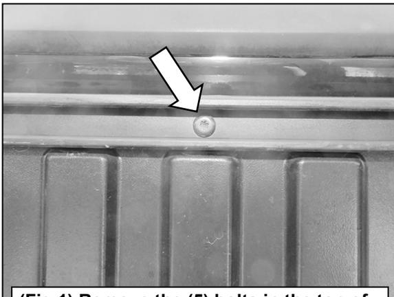
**(Fig 1) Remove the (5) bolts in the top of the bed, place the bolts in a safe location**
