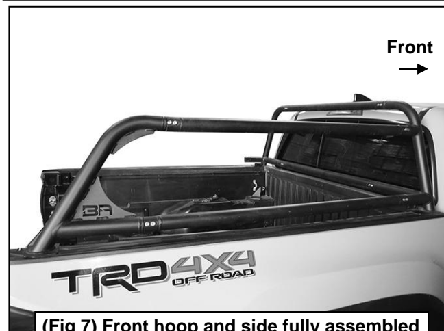
(Fig 7) Front hoop and side fully assembled (passenger/right side pictured)
