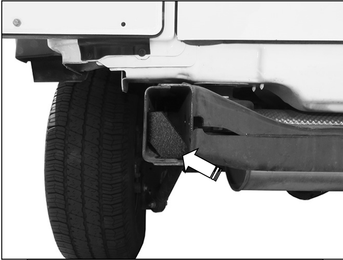
(Fig 5) Insert 14mm Double Nut Plate into open end of frame (driver/left side pictured)
