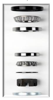
Installation order of bearings in swing arm barrel
