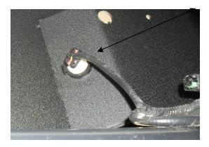
4 Install d-rings plate using supplied hardware.
