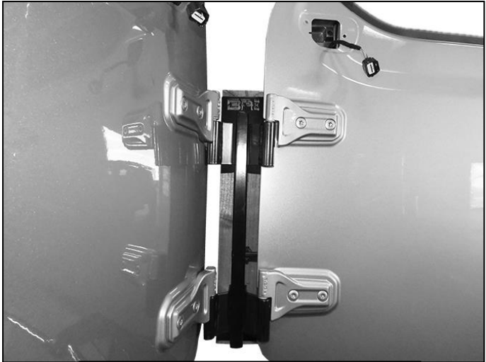
(Fig 9) Bushings and doors installed
