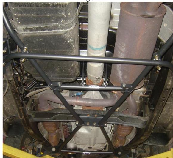
Complete Install w/Driveshaft Safety Loop option
