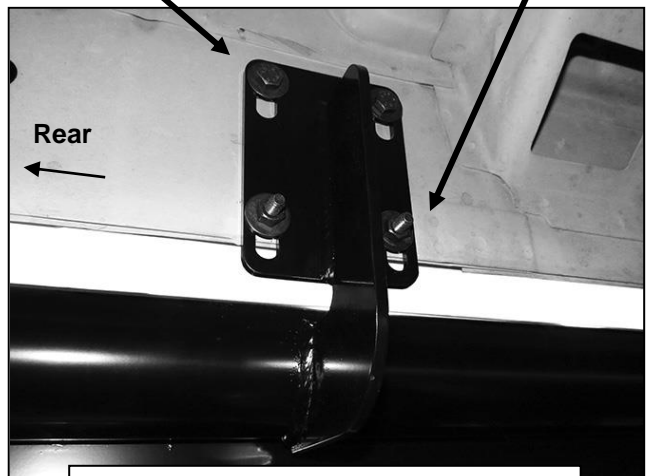
(Fig 7) Driver/left rear mount installed
