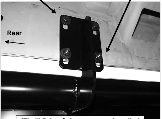
(Fig 7) Driver/left rear mount installed
