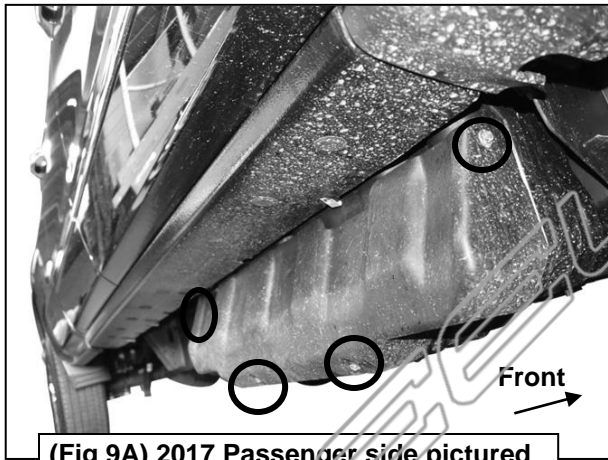
(Fig 9A) 2017 Passenger side pictured with DEF plastic tank cover. Remove (4) hex bolts to remove plastic cover
