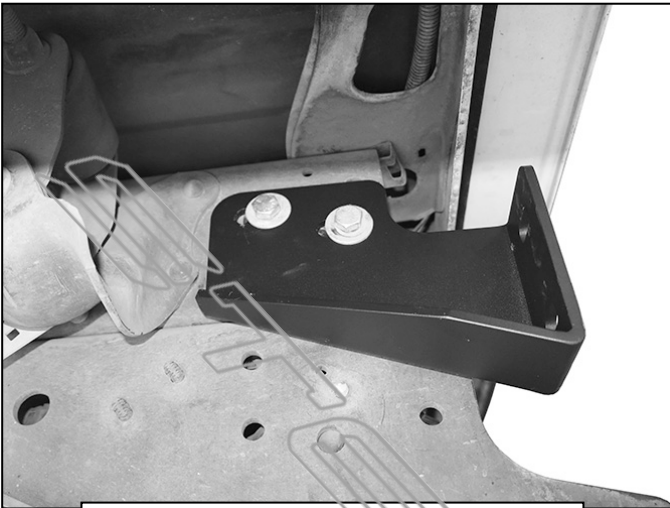
(Fig 3) Reuse the factory hardware to attach the driver/left Frame Mounting Bracket to the side of the frame
