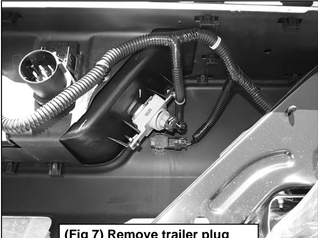
(Fig 7) Remove trailer plug and unplug license plate light
