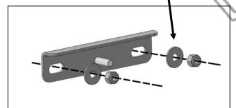
(Fig 5) Attach (1) Support Bracket to the threaded studs
