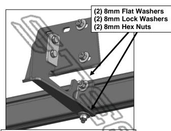
(Fig 13) Attach the Universal Mounting Tube to the Front Mounting Brackets.
