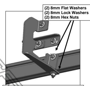
(Fig 14) Attach the Universal Mounting Tube to the Center Mounting Brackets.
