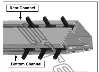
(Fig 8) Insert T-bolts into the rear and bottom channels on the universal mounting tube.
