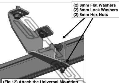
(Fig 12) Attach the Universal Mounting Tube to the Front Mounting Brackets.
