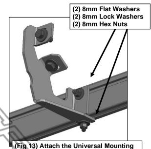
Tube to the Center Mounting Brackets.
