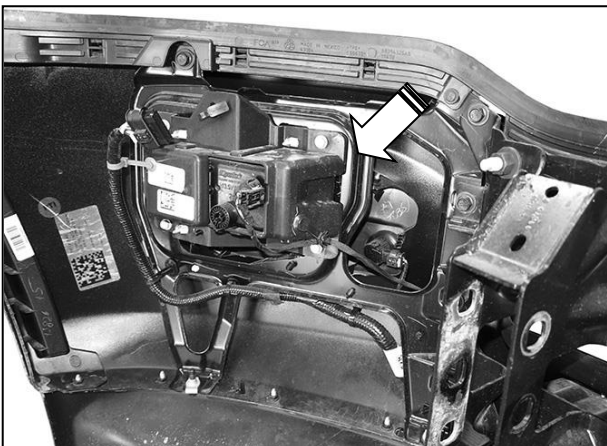
(Fig 9) Remove the wiring harness, sensors and fog light assemblies from bumper (if equipped)
