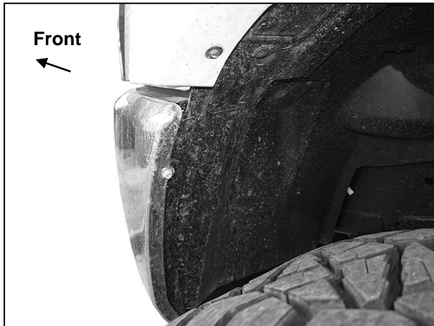
(Fig 1) Remove screws attaching ends of bumper to fender liners
