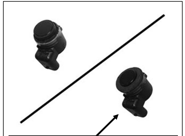
(Fig 11) Remove silicone seal from sensor. Slide large Seal over end of sensor (arrow)
