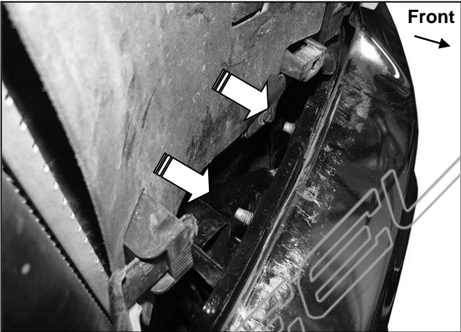
(Fig 3) Remove driver side top bumper hardware
