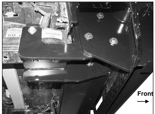
(Fig 12) Passenger/right side of Bumper attached to Bracket assembly, (pictured from behind and below Bumper)
