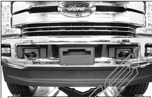
(Fig 3) Remove plastic air dam from bumper
