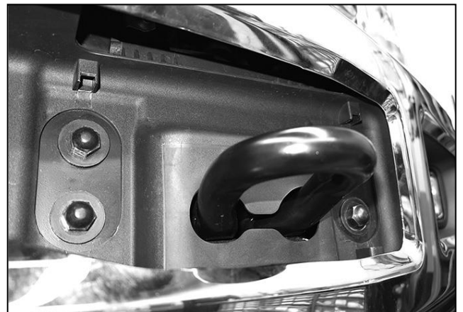
(Fig 6) Remove bumper bolts (driver side pictured)
