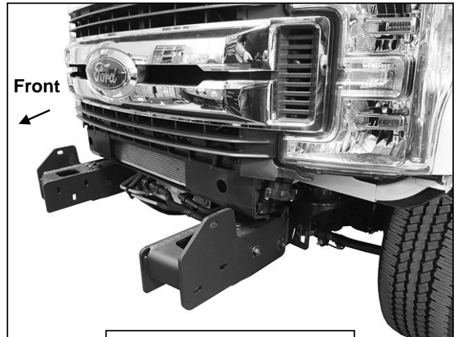
(Fig 10) Brackets installed
