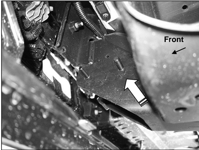
(Fig 9) Insert Double Bolt Plate through holes in outer side of frame (arrow)
