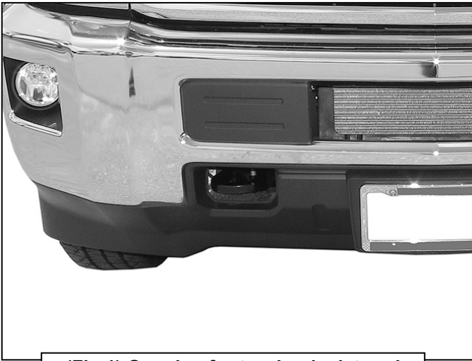
(Fig 1) Opening for tow hook pictured
