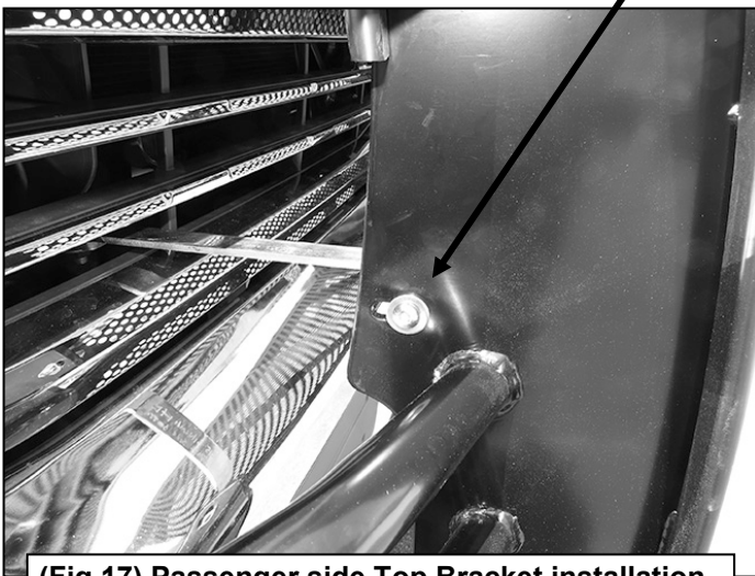
(Fig 17) Passenger side Top Bracket installation pictured. Adjust position so that Bracket cannot come in contact with plastic grille
