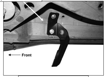
(Fig 4) Passenger/right front Bracket
