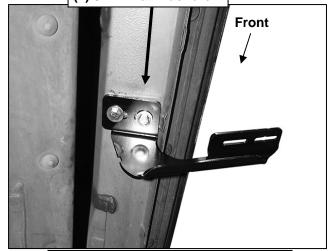
(Fig 6) Passenger/center mounting Bracket installed (note notch)
