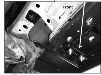
(Fig 10) Passenger/right front Bracket
