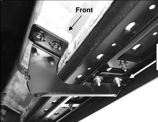
(Fig 11) Passenger/right center Bracket
