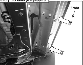
(Fig 1) Passenger/right front and center mounting location
