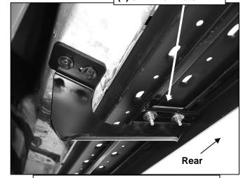
(Fig 12) Passenger/right rear Bracket
