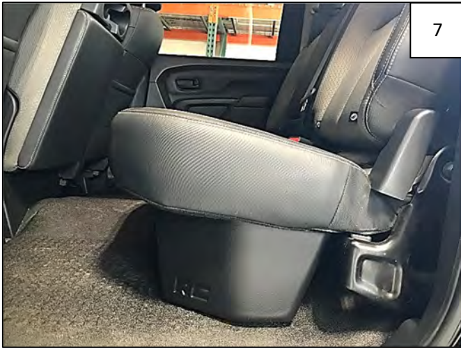
Completed Underseat Storage Installation.
