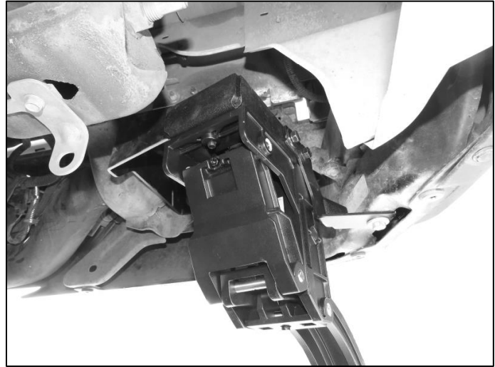
(Fig 8) Attached Base Arm and Bumper Support Bracket
